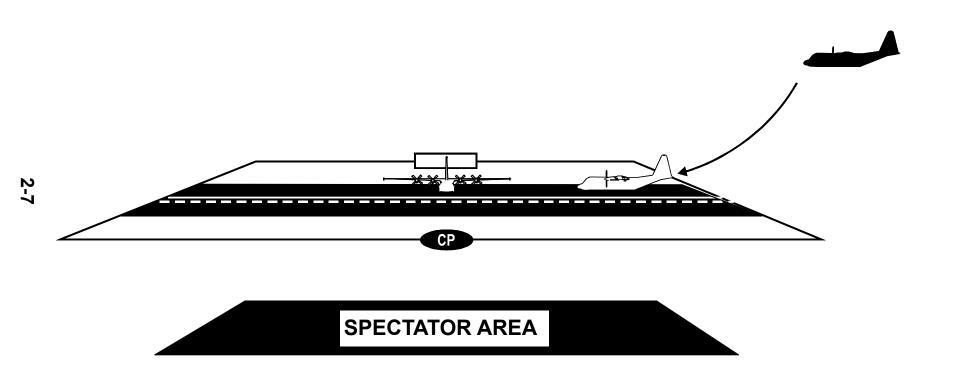
MANEUVER: Behind the crowd, the landing gear/flaps will be lowered and a turn back towards the show line will be commenced, rolling out on runway centerline at 1000-1200' AGL. As the intended point of landing is approached, a 20°-25° nose-down approach will be commenced. After landing, the aircraft will back up, face the crowd line, and exit the runway.
