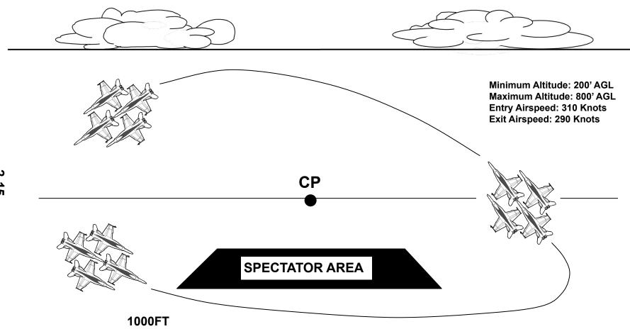
MANEUVER: In Diamond formation the Diamond executes a non-aerobatic right to left circular pass at less than 60° AOB crossing over CP at a minimum ALT of 200'.
