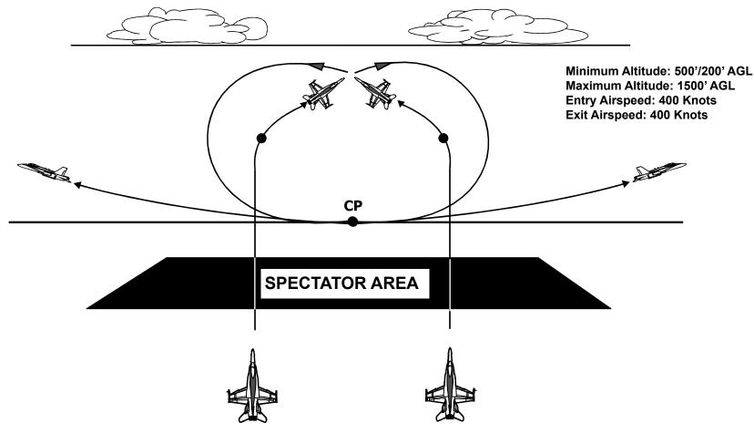
NOTE: Low show clear is 20° nose up and 2 1/2 rolls. Flat show clear is 10° nose up and 1 1/2 rolls.
