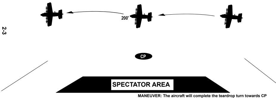
MANEUVER: The aircraft will complete the teardrop turn towards CP using the 30° ingress line. Once established on the 30° ingress line, a descent from 500' AGL to 200' AGL will be made. Abeam the crowd line, a roll into a 60° AOB turn towards will be performed. The turn will be continued to depart on the 30° egress line. Abeam the crowd line on the 30° egress line, wings will be leveled and a 10° nose-up climb will be initiated to 1200' AGL.
