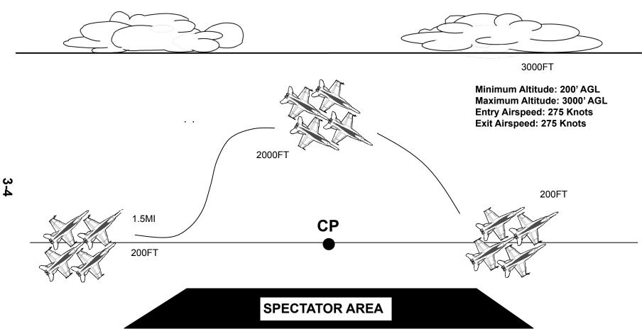
MANEUVER: Approaching CP in Diamond with Landing Gear extended, all four aircraft roll 360° in formation, starting the roll at 1200' to apex at approximately 2000'. Minimum altitude on the ingress and egress roll line is 200'.
