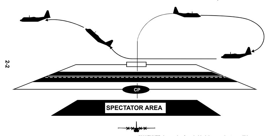
MANEUVER: Ingressing from behind the crowd, a turn will be commenced at CP to establish a 1000' AGL downwind position. The aircraft will then commence a descending turn back to the show line. Abeam CP on the 500' line at 100' AGL, the aircraft will commence a 45° nose-up climb to level off at 1000-1800' AGL.
