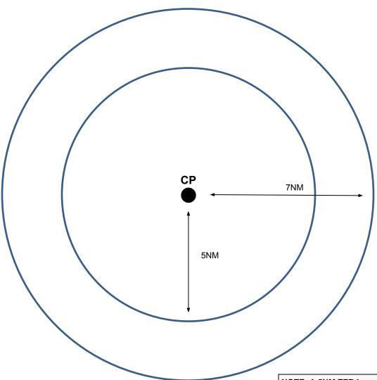
NOTE: A 5NM TFR is required for all flight demonstrations. A 7NM TFR is required for all demonstrations where the density altitude is expected to be greater than 4,000FT at the time of the demonstration.
