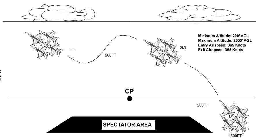
MANEUVER: Approaching CP in Diamond, all four aircraft roll 360° in formation, starting the roll at 1500' and topping at approximately 3200'. Minimum altitude on the ingress and egress roll line is 200'.
