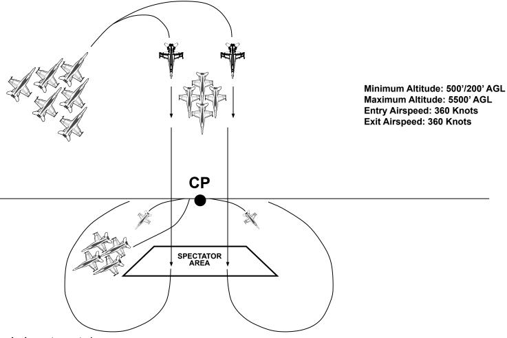
NOTE: This maneuver is done at remote / over water show sites and in Low / Flat Shows where Diamond Burner Loop on takeoff and Low Transition / Split S on takeoff are not conducted.
