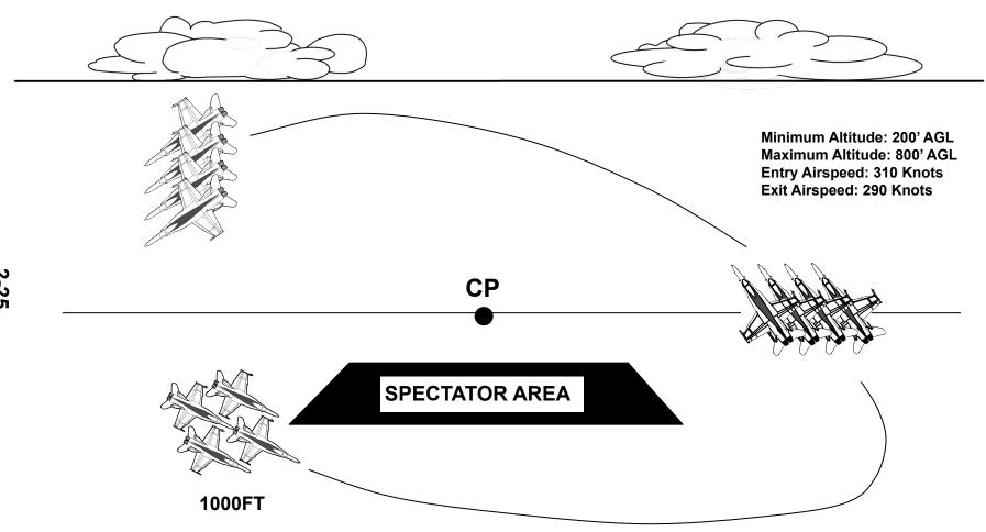
MANEUVER: In right Echelon the Diamond executes a right to left non-aerobatic circular pass at approximately 60° AOB crossing over CP at a minimum altitude of 200'.
