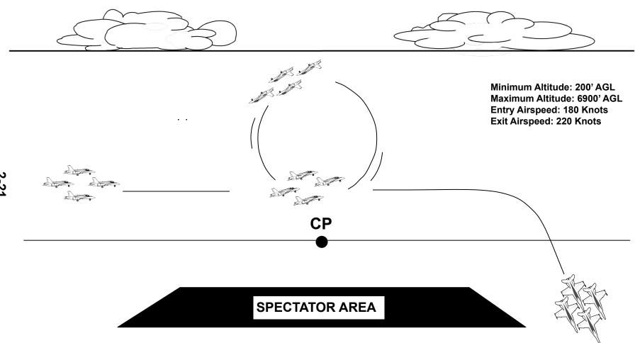
MANEUVER: In the Diamond formation all four aircraft will complete a loop over CP on the show line with the landing gear and hooks extended.
