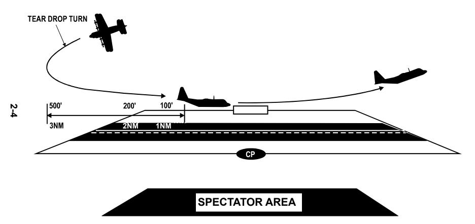
MANEUVER: The aircraft will make a teardrop turn back toward the show line to position itself on the 500' line. Abeam CP at 50' AGL, a climbing turn will be commenced away from the crowd to set up for the head on pass.
