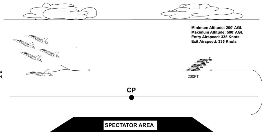
MANEUVER: At approximately 3 NM, aircraft #1,2,3,4 and 5 transition to a Line Abreast formation leveling off at 200' AGL on the 500' Show Line. Egressing crowd left, aircraft #1-4 shift back to Diamond and detach #5.
